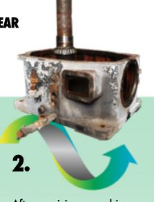
After receiving your drive, an Amarillo® Gear Technician will inspect for wear and damage. Many times there are parts that can be cleaned and reused providing you, the customer, with considerable cost savings. You will then receive an As Found Condition Report, photographs and an updated quote.
